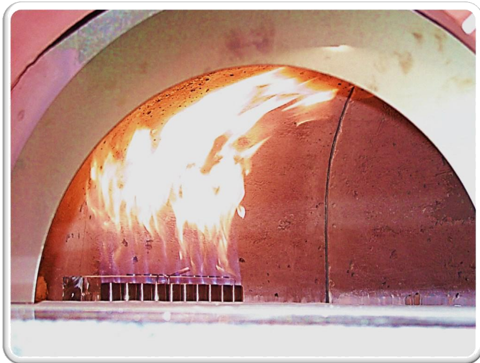
Image of the flame on maximum with power 70% and temperature 420°C
